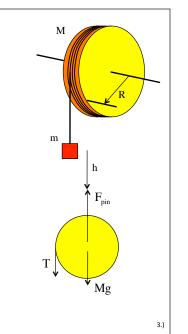
NOTE: A dumb but common error is to short-cut the process by looking at the f.b.d. and jumping to the conclusion that the tension T = mg. It isn't if there is acceleration in the mix! Noting that the acceleration is downward in the direction I normally define as negative (hence the need to unembed the negative sign associated with the "a" term), the process yields:
